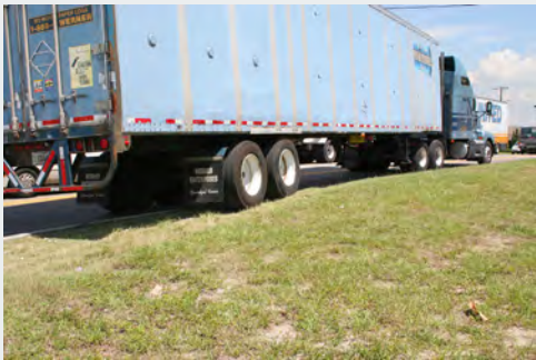
In low activity areas, some use of the shoulder may be appropriate where turns across the shoulder are infrequent, pedestrian volumes are low, and the roadway base is designed to accommodate occasional loads.
