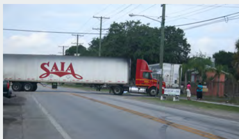
The slower acceleration rates for trucks are particularly important considerations at unsignalized intersections with significant cross-street goods movement activity.
